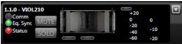
**Comm:** Green indicates that communication between speaker and Control is working. In case of communication error the indicator becomes red.
