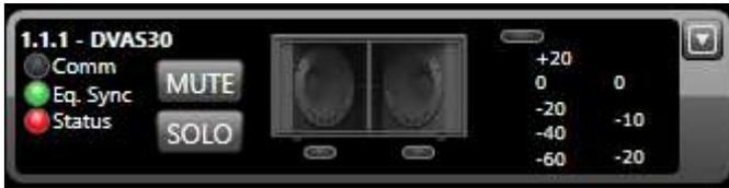
**Comm:** Green indicates that communication between speaker and Control is working. In case of communication error the indicator becomes red.
