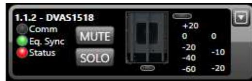
**Comm:** Green indicates that communication between speaker and Control is working. In case of communication error the indicator becomes red.
