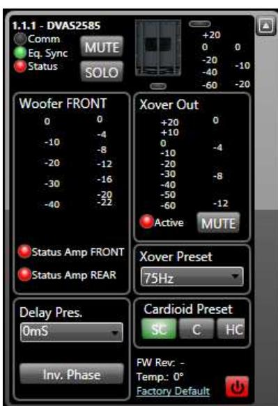
**Woofer Front - Xover Out Panels:** show advanced parameters for each audio way (Main Woofer and Xover Out).
