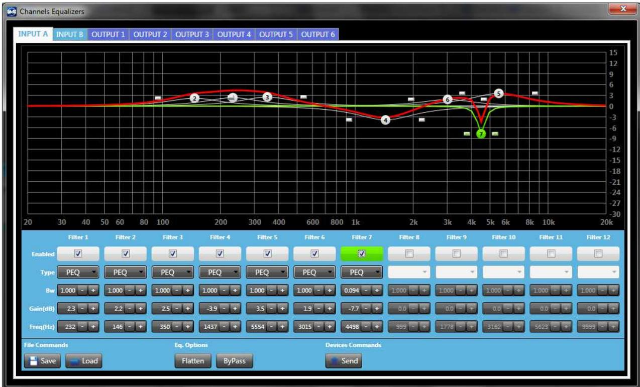
PEQ panel allows to equalize each single Input or Output channel, correcting one or more frequencies that have to be reduced or increased.
