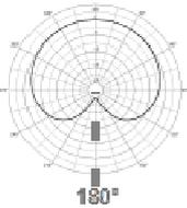
C = Cardioid (heart shaped diagram). Rear attenuation range is 180° (in line with the front). This configuration is to be used if the speaker is placed in front of the stage in a central position; in this case the low frequencies are practically eliminated on stage.
