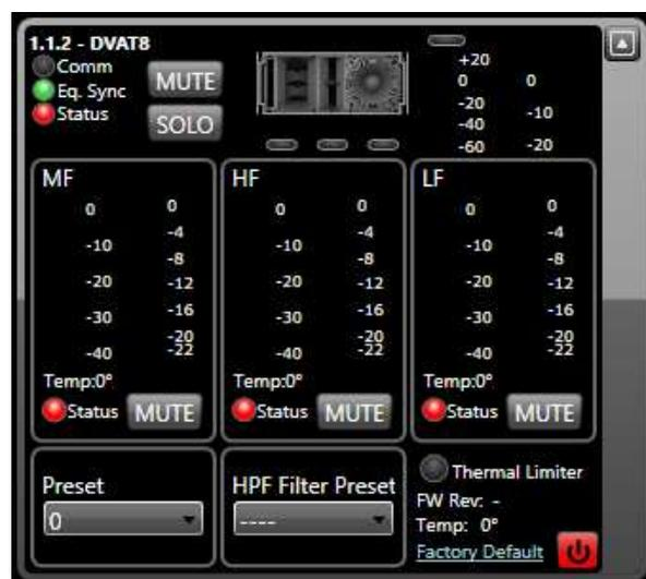
**MF-HF-LF Panels:** show advanced parameters for each audio way (Midrange, Tweeter and Woofer).
