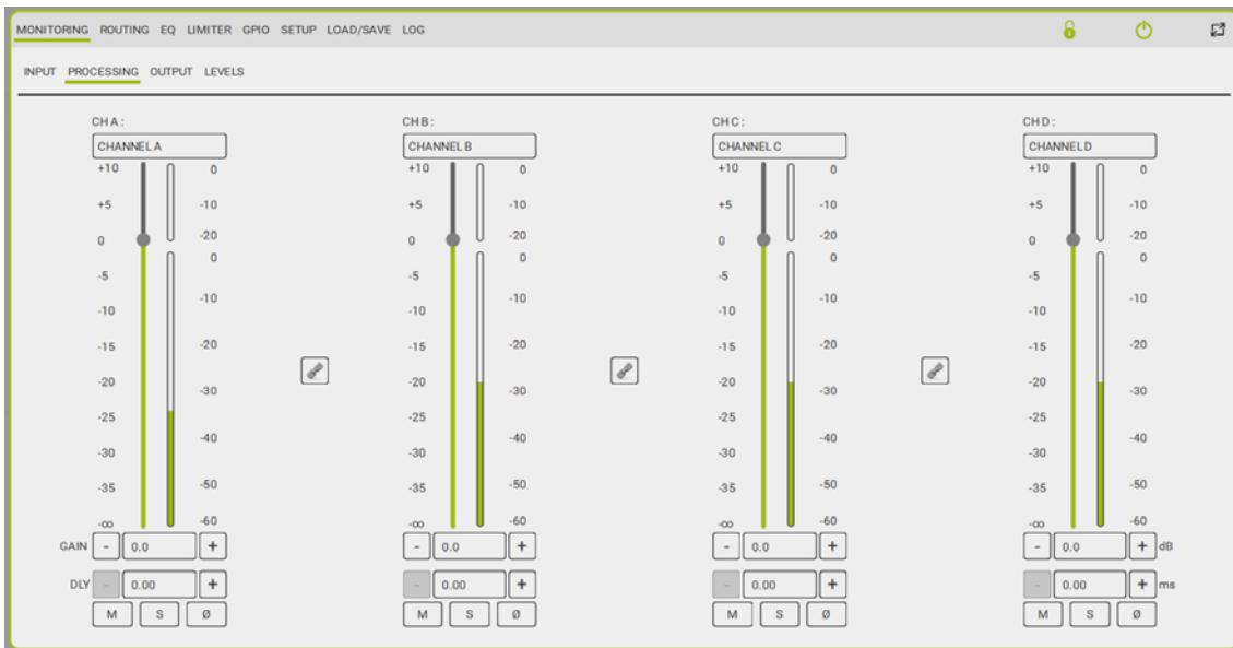
From the Processing section, you can monitor the signal levels and compression in the processing channels, solo, mute, invert the polarity, apply a delay and link channels A-B, B-C and C-D. The Link control affects the entire processing chain. The compressor meter refers to the compressor enabled in the Limiter => Processing Channels section.
