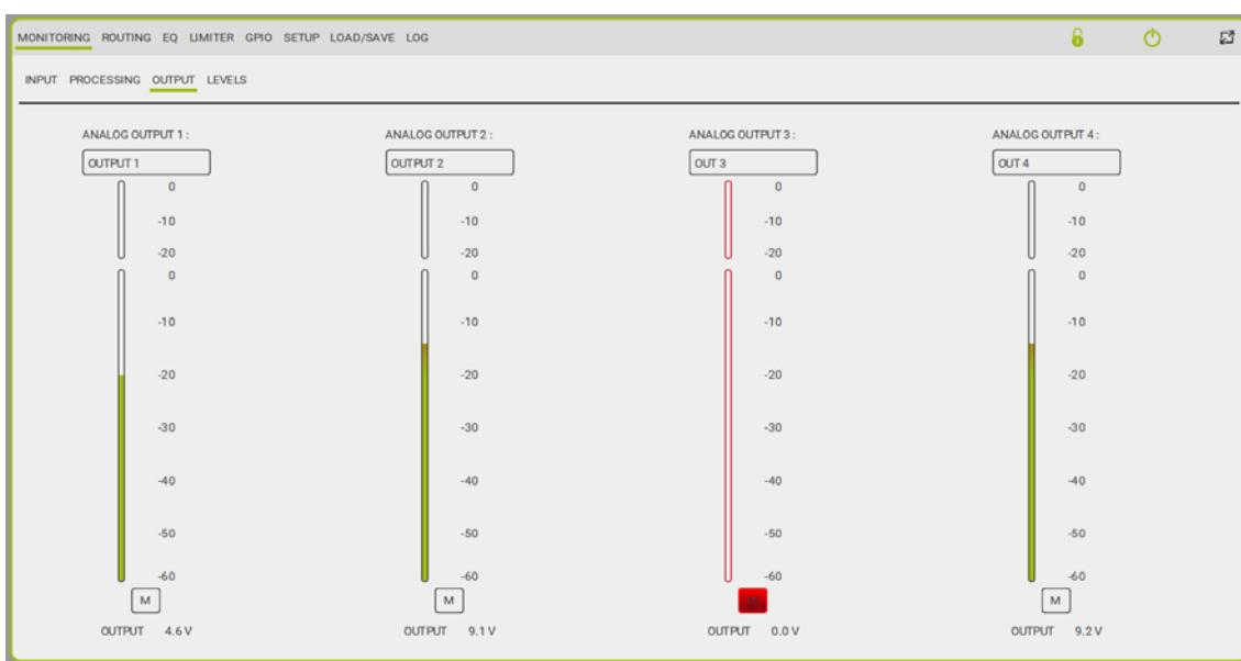
From the Output section, you can view the amplifier output levels, the total compression, and mute the single channels.
