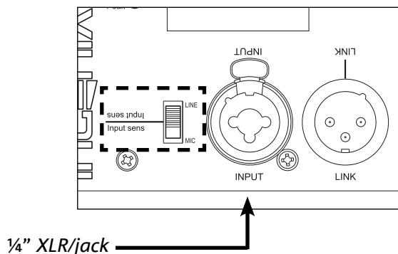
To connect 2 or more speakers to the same audio source in certain installations, you may find it convenient to daisy chain the signal from a first module to the next and so on. First, connect an audio source to the INPUT of the first speaker. Then connect the LINK output of the first loudspeaker to the INPUT of the second speaker with a balanced XLR cable. This second operation can then be repeated by connecting loudspeakers to achieve the most suitable installation for the setting.
