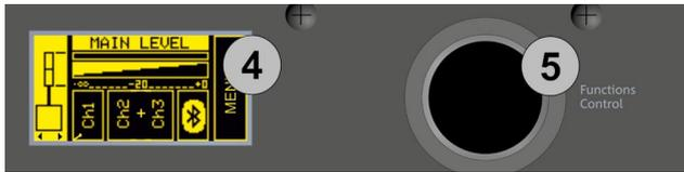
You can view and configure the various ES503 system parameters using the OLED screen [4] and the rotary button [5] in the Functions Control section.
