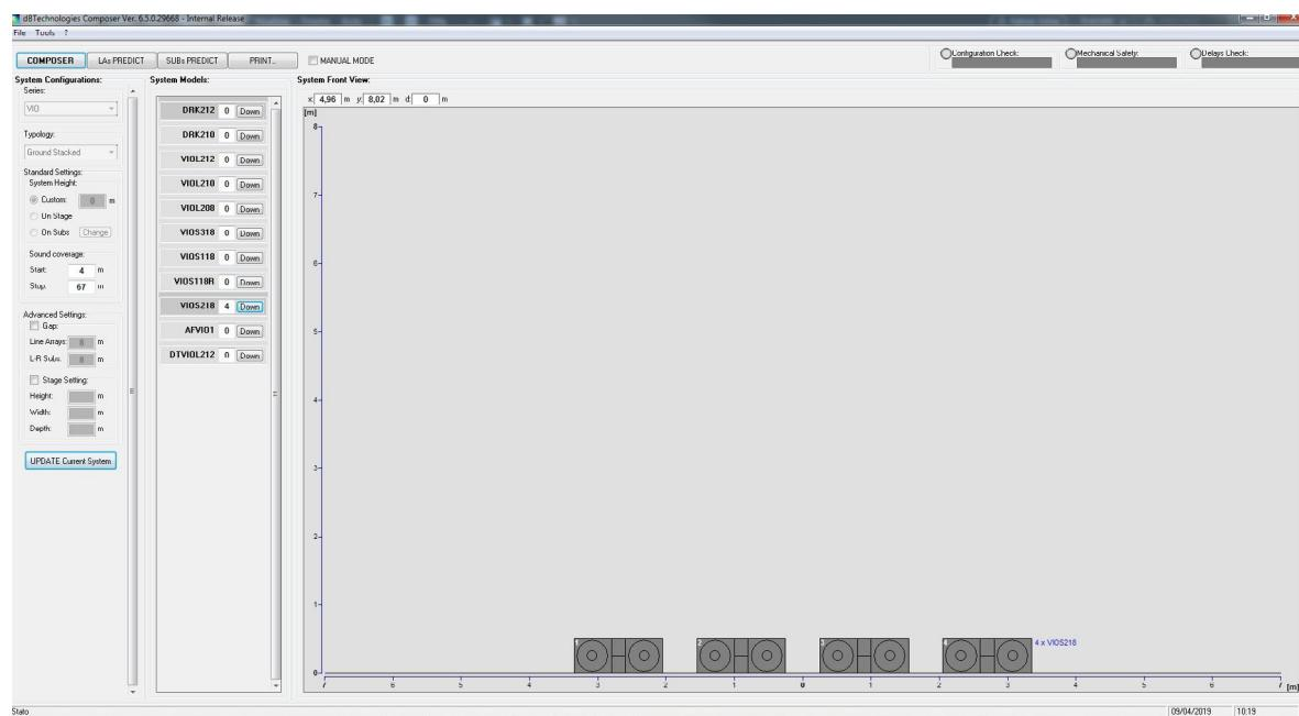
To achieve a predictive simulation, enter all system main design parameters in the COMPOSER section. The SUBs PREDICT sub page suggests: the angle of the different modules and the different parameters relating to the control section, such as delay, polarity, crossover frequency. In addition, a message relating to installation safety appears inside the "Mechanical Safety" box. Use these data to configure the control parameters on the subwoofer panel.
