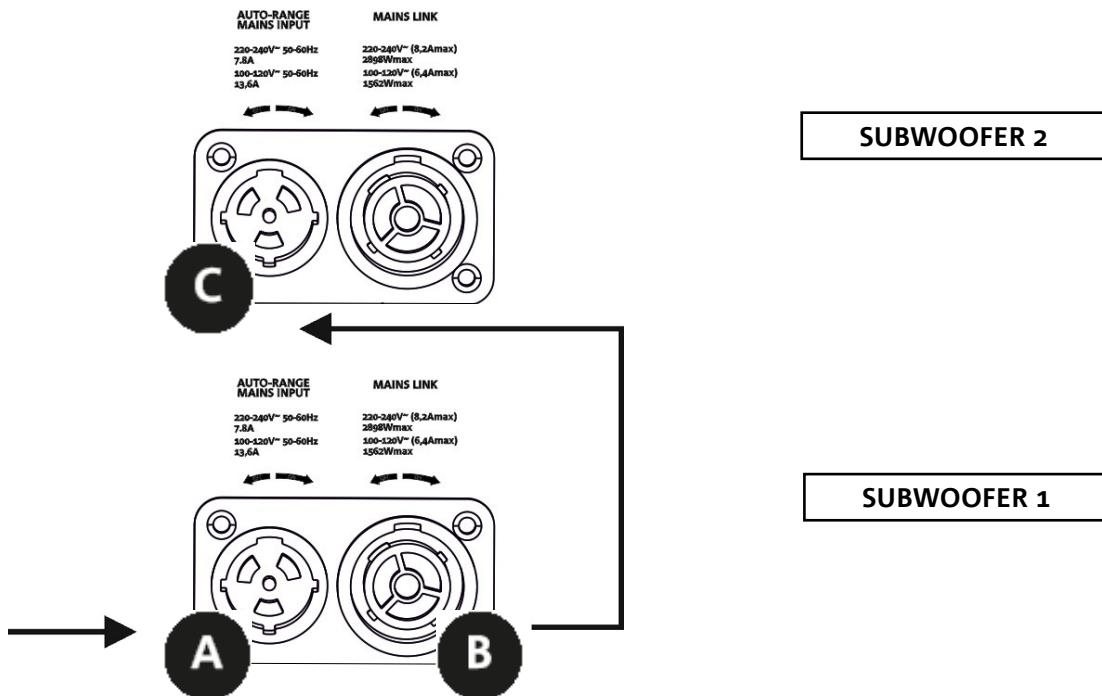
The figure above shows a general connection where a subwoofer 1 is under subwoofer 2. To this end, use cables with powerCON TRUE1® connectors (only one power cable is supplied with the package).
