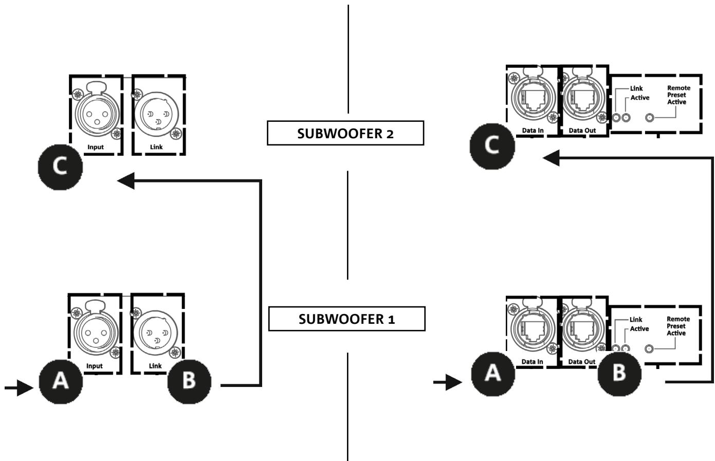
The figure above shows a general connection where a subwoofer 1 is under subwoofer 2 as well as the audio and network connections. To this end, use the not supplied cables with XLR (audio) and etherCON/RJ45 (network) connectors. For further information on the available types of cables, refer also to the image in next page.
