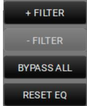
Buttons to add or remove a filter, or bypass or reset all filters.
