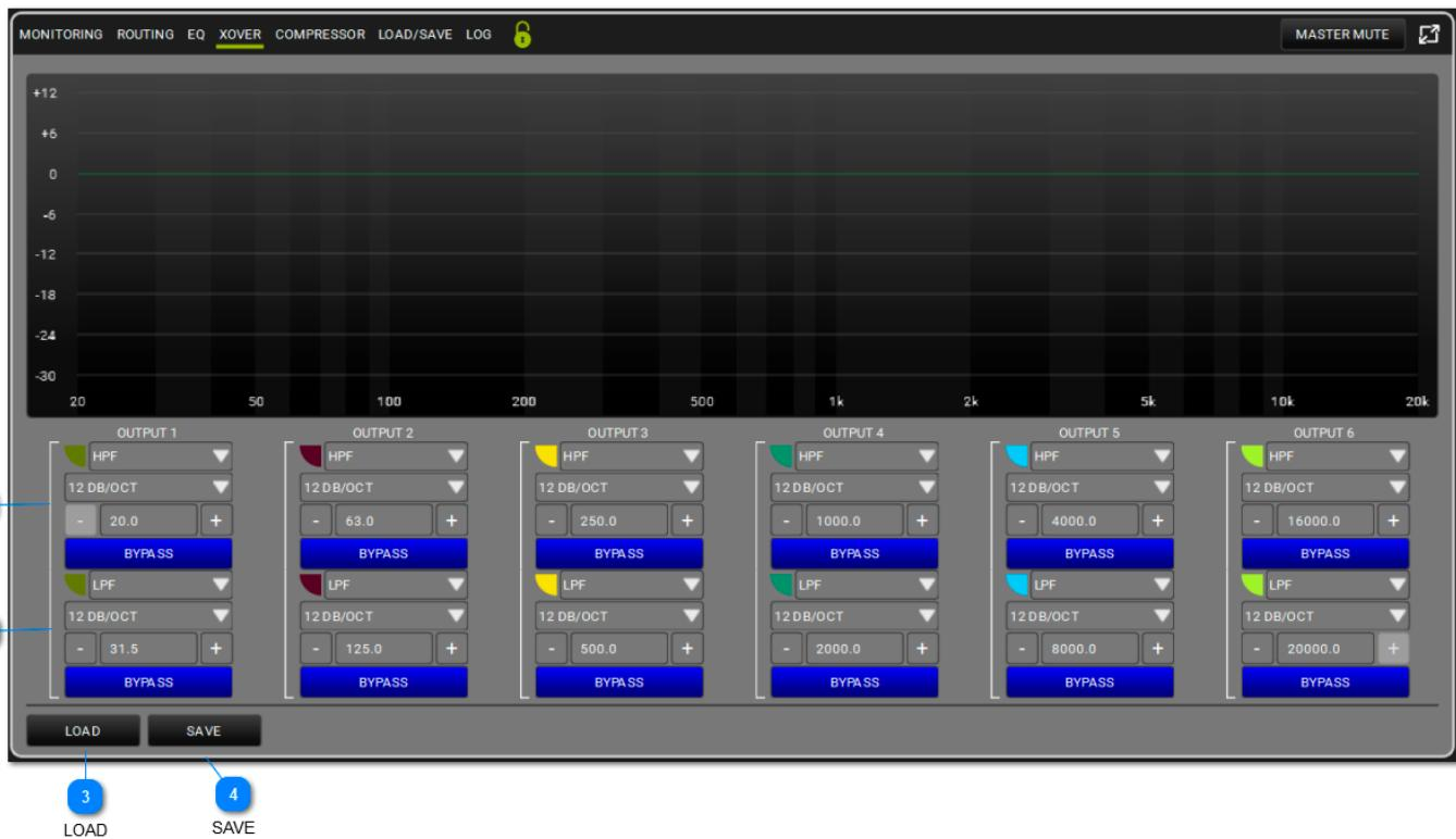
For each output channel you can set an HPF and LPF filter to shape the crossover point, by selecting frequencies and slopes. Each filter can be bypassed to appreciate the difference with or without it. You can also save or load pre-sets. Please note that you can assign a colour to each filter, for a clearer display.
