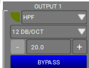
You can choose between High Pass Filter or Low Pass Filter and select the slope (12/24/48 dB/OCT) and the cut-off frequency.
