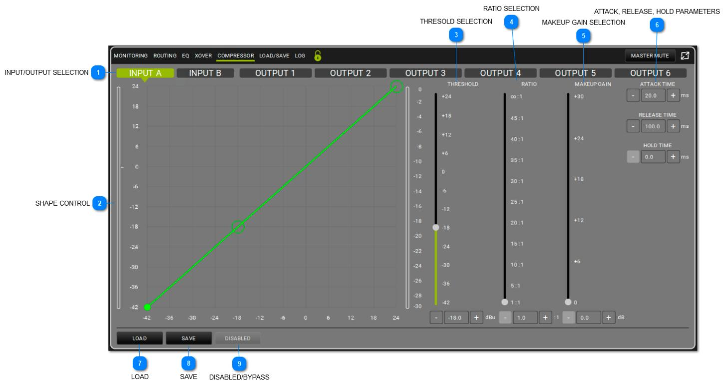
This applies a compressor to the selected channel. The shape (in terms of threshold and ratio) can be controlled either in the graphic or with the cursors.
