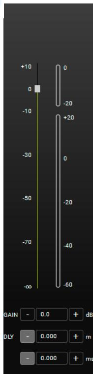
The LEVEL/DELAY WINDOW allows you to immediately view and control the levels, gain and delay in a group.
