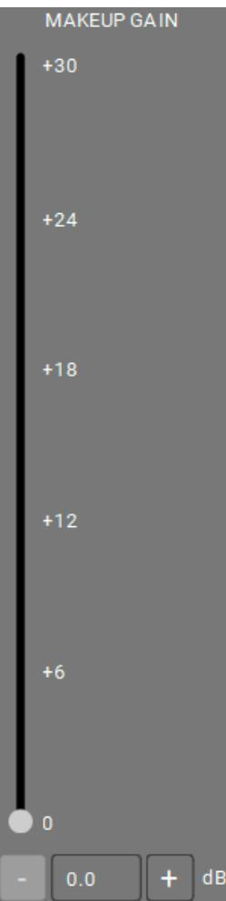
It defines the gain to be applied to the signal processed by compression
