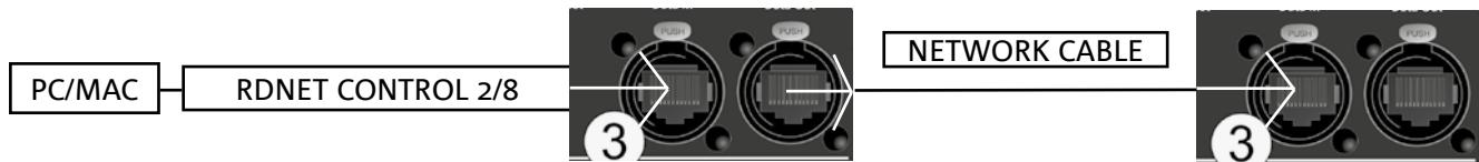
To enable remote control, connect the Data Input of the first speaker to the hardware interface (RDNet Control 2 or RDNet Control 8) using cables fitted with eternCON connectors. Then connect the Data Output of the first speaker to the Data Input of the second, and so on. When the speakers are powered on, the Link LEDs illuminate to indicate the connection has been made. The other Active LEDs will start flashing to indicate the presence of data traffic.
