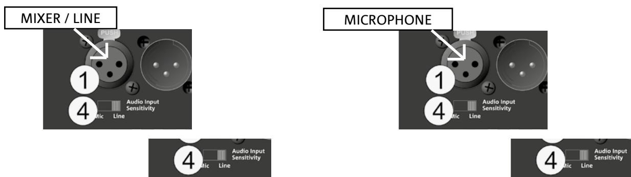
Connect the audio source to the input 1 in the input and control section at the back of the speaker. In particular, in case of using a microphone, set switch 4 to "MIC".
