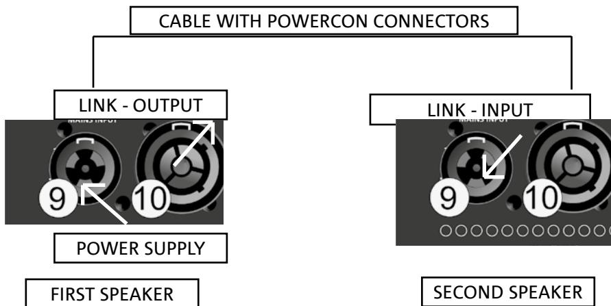
On the VIO X you can link the power supply from the first speaker to the next. To link the power supply in this way, simply connect the power cable supplied to the MAINS INPUT on the first VIO X speaker and connect a second cable with suitable connectors (optional) between the MAINS LINK output and the MAINS INPUT of the next VIO X speaker. This type of connection can be repeated up until the maximum permissible current is reached and indicated in the MAINS LINK connector of the first speaker.
