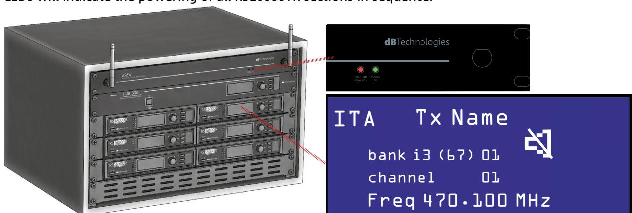
c) on the front side, the AS6W LEDs indicate that the antennae are powered. The displays will light up. In particular, those of the RS16000R receivers show a screen similar to that shown in the figure.
