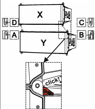
Please note that the SAFETY LOCK, once it is necessary to disassemble two modules, must be pulled up to unlock them.
