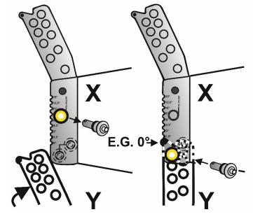
CHECK PERIODICALLY THE INTEGRITY AND THE FUNCTIONALITY OF THE ENCLOSURE, OF THE PINS AND OF THE BRACKETS, FOR A SAFE INSTALLATION. MAKE SURE THAT THE PINS SECURE PROPERLY THE MODULES AND THAT THEY ARE FULLY LOCKED.
