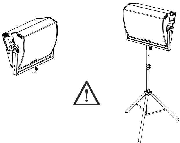
The SA-WT stand adapter allows you to install a VIO W15T speaker on a tripod (D=35mm) or on a subwoofer using a pole (D=35mm). The maximum allowed height of the base of the adapter above the floor is 150 cm.
