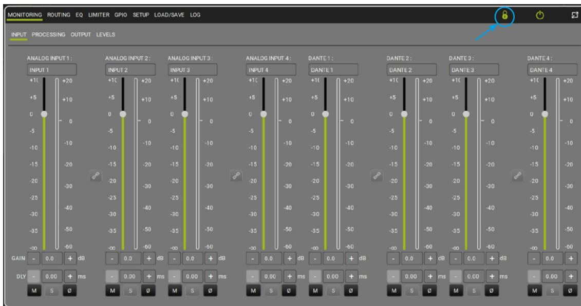
To open the Lock Device window, press the padlock at the top right of the main Aurora screen. You can lock/unlock Aurora pages from here.
