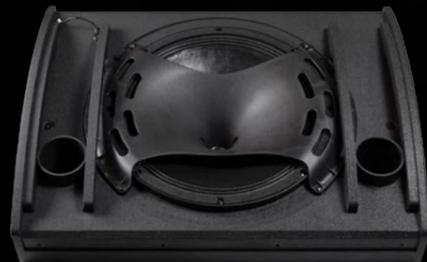
VIO W15T is equipped with a coaxial component encompassing a 15" neodymium woofer and a 3" neodymium driver. HF reproduction is routed through a horn allowing for a sharp 80x60° dispersion pattern.
