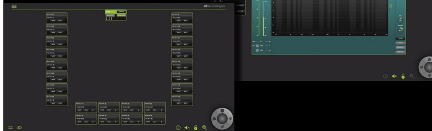
Cross-platform developed (Win, Mac OSX) by dBTechnologies Software Department in order to guarantee maximum reliability, Aurora Net works via Ethernet cable (or alternatively via XLR), allowing for an advanced, completely customizable DSP control and DIGITAL Audio management (via Dante™ protocol) on the same cable.
