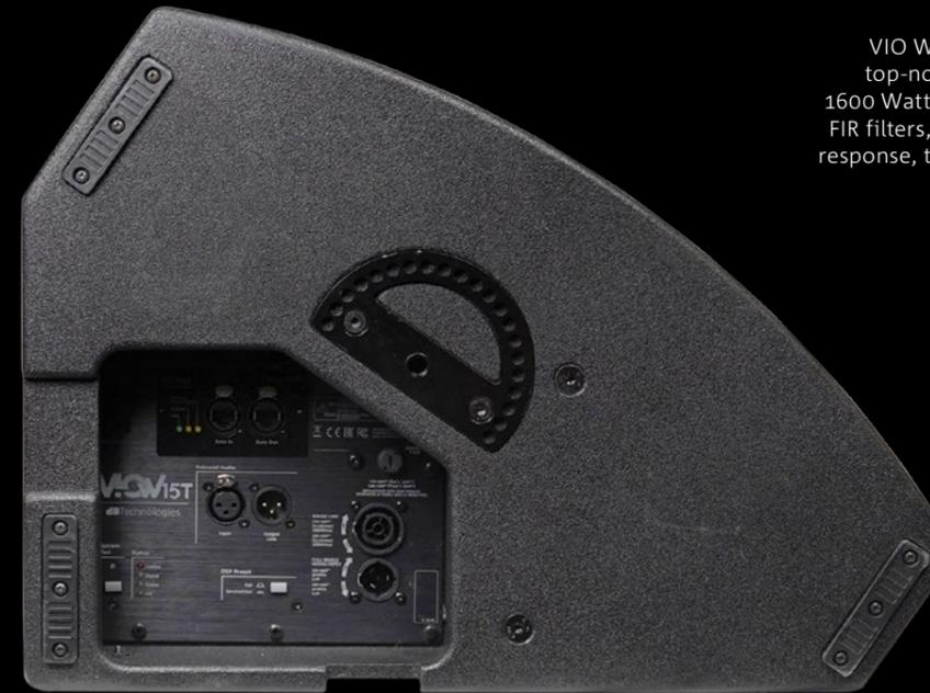
VIO W15T is a self-powered box, equipped with a top-notch class D Digipro G4 amplifier, delivering 1600 Watts RMS. Its powerful DSP takes advantage of FIR filters, allowing for very flat frequency and phase response, together with great feedback rejection, and impressive SPL capability up to 137 dB.
