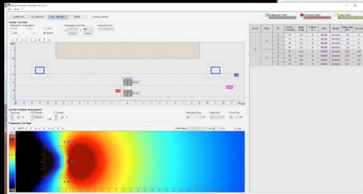
Furthermore the software allows the user to predict acoustic coverage of both tops and subs, splay angles and it automatically checks the set up presets in order to evaluate the efficiency of the system and its nominal coverage.
