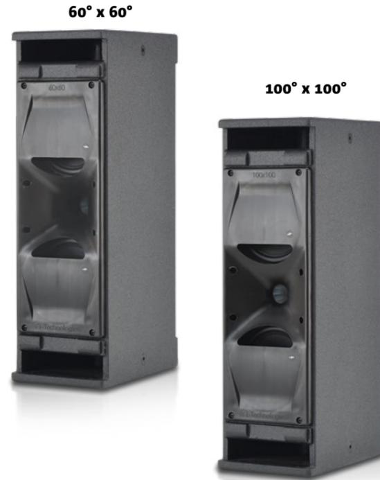
VIO X205 is a 2-way speaker equipped with 2x5" (1" voice coil) and 1x1" driver (1.4" voice coil). The 400 W RMS DigiproG3 amplifier powers a cabinet able to deliver up to 126 dB despite its very compact dimensions: only 150 x 485 x 240 mm (WxHxD).
