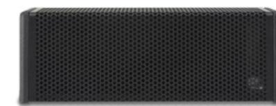
The 2-way system is equipped with 4x 4" neodymium HF speakers and 1x 10" woofer, placed in an exclusive anti-feedback acoustic configuration. The cabinet is driven by a 400 W RMS Digipro G3 amplifier and full remote control is enabled via RNet and Aurora Net software.
