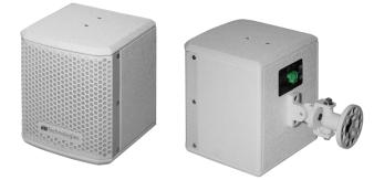
LVX P5 is a passive speaker equipped with a full-range single transducer (5" LF and 1" HF). The most efficient acoustic design, allowing an extended coverage pattern (135°x135°) and a vigorous SPL up to 115 dB, makes this mini full range system the perfect solution to render speech or background music in small venues.
